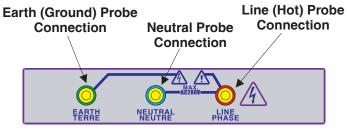
apply only Voltage Model @ 50Hz or 60 Hz. Voltage Model (Vac) A=240, B=230, C=220, D=110
