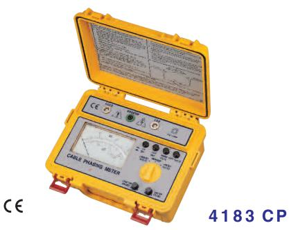
The **4183 CP** is a Cable Phasing Meter that offers a quick method of measuring voltage and determining phase rotation of underground distribution systems using the capacitive test point of elbow connectors. Most manufacturers of high voltage cable terminations incorporate capacitive test points in their elbow connectors. These test points are designed for measuring purposes.
